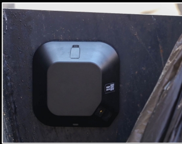
installed dumpster camera
